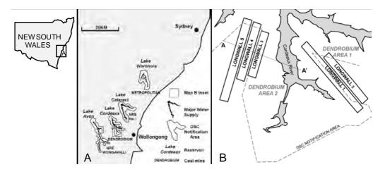
*Figure 1* A - Location of major water supplies South of Sydney; B - Dendrobium Mine illustrating location of longwalls 1—5 (LW1—5) and cross section A-A' Figure 3.
