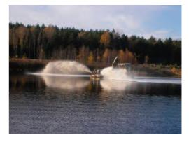
Figure 5 Spreading boat in action: A slurry of  $CaCO_3$  and lake water is prepared on the boat and distributed up to 25 m to each side of the boat. The boat distributes up to 250 tons  $CaCO_3$  per day.
