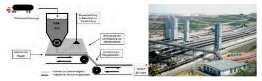
*Figure 2* Principle of limestone mixing with the overburden (left, Wisotzky 2003, P.51) and the four dosing stations in Garzweiler (right).
