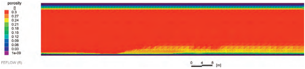
Figure 2 Exemplary result of a reduced porosity caused by chemical reactions and precipitation.
