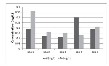
**Figure 4** Results of leachate tests for aluminum and iron concentrations (mg/L) of soil from five strip mined sites in the Middleton Run watershed.
