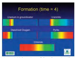
**Figure 1** Initial uranium roll-front formation. Flow is from left to right.
