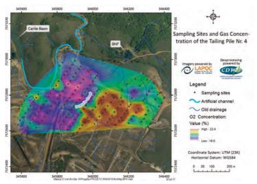
Figure 2 Gas concentration map for  $O_2$  at WRP4.
