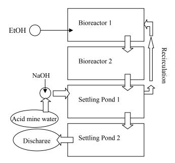
Figure 1. Constructed pond reactor system. Ponds have dimensions 10m x 3.5m x 3.5m deep; Bioreactor ponds are filled with 25 cm rock. Ethanol is provided at Bioreactor 1, NaOH is added to mine water just prior to entering Settling Pond 1, and water from Settling Pond 1 (neutral pH high in sulfate) is pumped to Bioreactor 1. Settling Pond 2 acts as a backup for sludge precipitation and storage. Water leaving Settling Pond 2 enters a basin prior to final discharge to the watershed.
