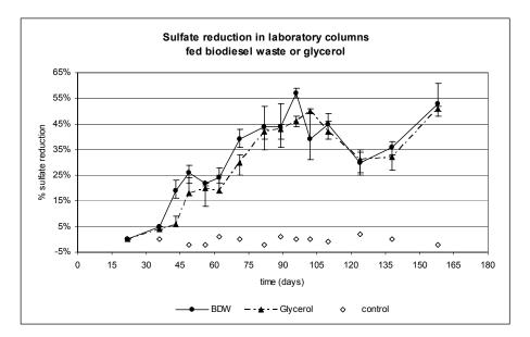
Figure 3. Columns fed biodiesel waste reduced more sulfate than columns fed glycerol, when bdw was provided in concentrations of glycerol equivalents to reduce 50% of influent sulfate water. The sharp decrease after day 105 occurred when columns were not fed enough iron, resulting in sulfide toxicity; when provided with iron after day 120, they recovered quickly.
