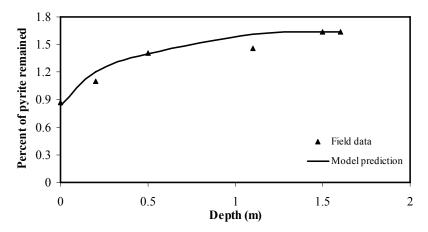
Figure 2. Comparison of the field data and modelling results of the percent of pyrite remained within the waste particles as a function of depth for sample No. 2.
