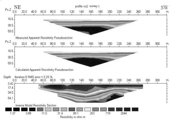
Figure 3. Inverse modelling results for geoelectrical data indicating measured apparent resistivity pseudosection, calculated apparent resistivity pseudosection and inverse model for profile number 2.
