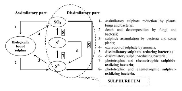
Figure 1. The biological sulphur cycle (Rehm and Reed, 1981; Luptakova et al., 2002).
