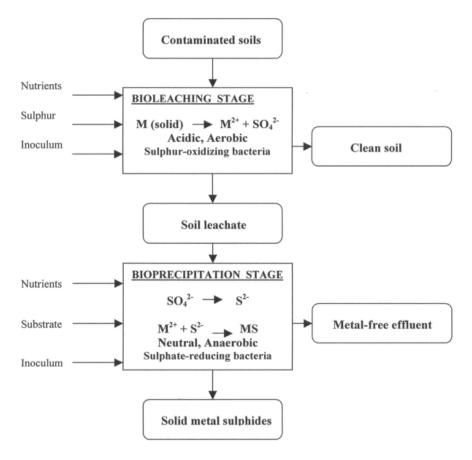
Figure 2. Diagram showing the integrated process for bioremediation of metal-contaminated soils (Eccles and Holroyd, 1996).
