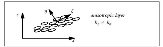
Figure 1. An anisotropic non-horizontal layered soil 2D model.
