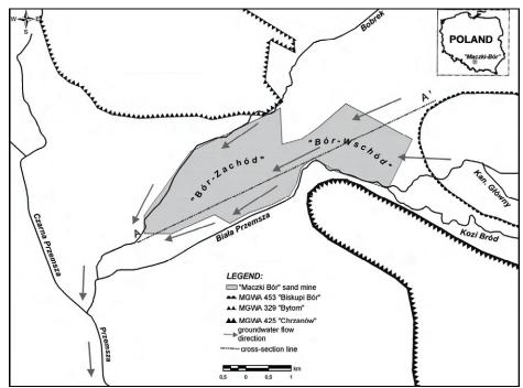
Figure 3. The expected groundwater flow directions in the vicinity of "Maczki-Bór" sand mine after finishing the dewatering.
