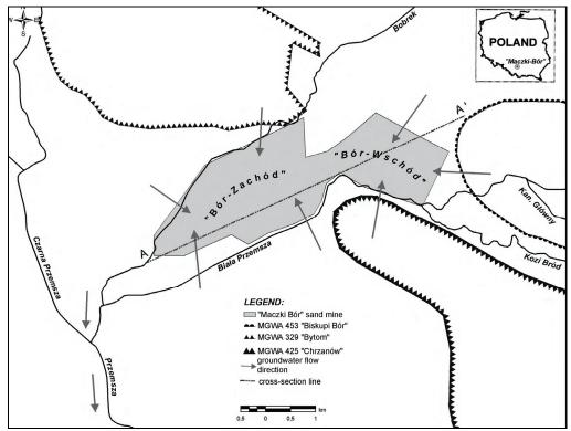
Figure 1. The groundwater flow directions in the vicinity of "Maczki-Bór" sand mine. Current situation.
