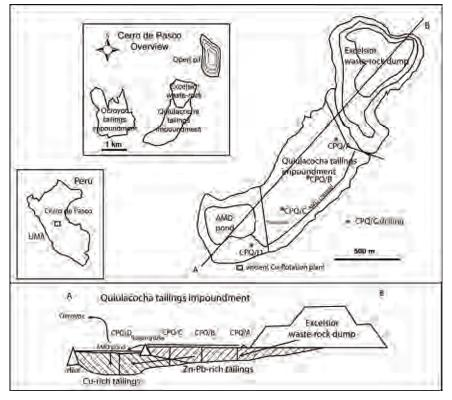
Figure 2. Location map of the open pit, waste-rock dump and tailings impoundments at Cerro de Pasco, Peru. The Quiulacocha tailings cover 114 ha, comprising 79 Mt of tailings, which contain ~ 50 wt% pyrite. The tailings are located at 4340 m altitude in a tropical puna climate with about 1025 mm/a rainfall. The tailings are partially overlain by the Excelsior waste-rock dump, which contains about 26,400,000 m<sup>3</sup> of
