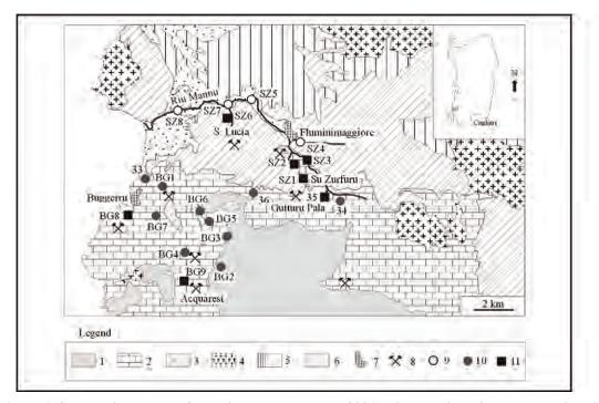
Figure 1. Schematic geology of Fluminese (Barca et al., 2001) with location of water sampling sites. Legend: 1. Lower Cambrian sandstone; 2. Lower Cambrian limestone-dolostone; 3. Upper Cambrian-Ordovician metasiltstone-metasandstone; 4. Hercynian granitic rocks; 5. San Vito Formation; 6. Tertiary-Quaternary sediments; 7. Town; 8. Significant abandoned mines; 9. Stream samples; 10. Spring and well samples; 11. Mine water samples.
