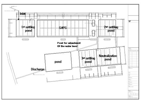
Figure 1. Plan view of existing passive treatment system.
