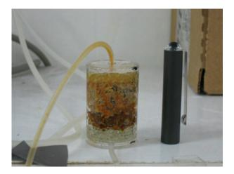
Figure 5. New experimental columns. The reactive part of the column is 2.5 cm in height and 2.6 cm in diameter.
