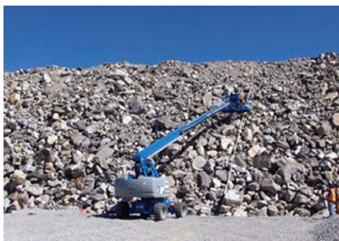
Figure 2. Photo showing waste rock sampling procedure at the tip face. Four tip faces were be sampled for each pile.
