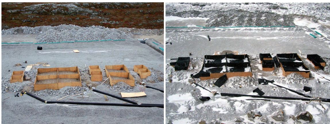
Figure 5. Photo to the left shows three lysimeter clusters constructed over the Type III test pad. Loops of wire on the lysimeter pads are heat trace cable. The black 25.4 cm insulated pipe house the 3.8 cm drainage pipes exiting from each lysimeter. The photo to the right shows a completed cluster lysimeters with an impermeable HDPE liner.
