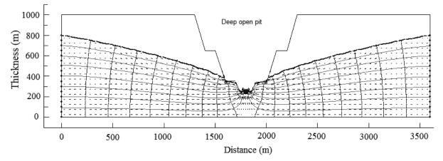
Figure 4. The results of two-dimensional modelling for a deep open pit mine in an unconfined aquifer.
