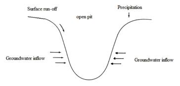
Figure 1. Inflow components into an open pit.
