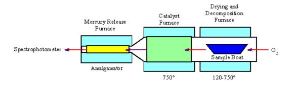
Figure 1: Schematic diagram of the mercury specific analyser DMA-80
