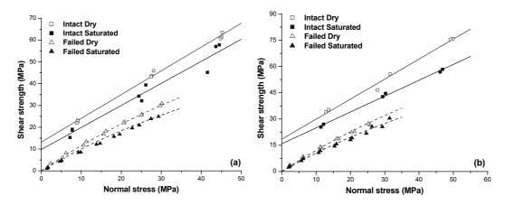
Figure 4: Strength envelopes of intact and failed (a) Coarse grained sandstone (b) Silty sandstone when dried and saturated
