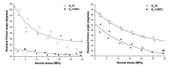
Figure 5: Developing tendency of the residual friction angle due to water, (a) Coarse grained sandstone (b) Silty sandstone
