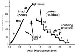
Figure 3: The multistage triaxial compressive testing method
