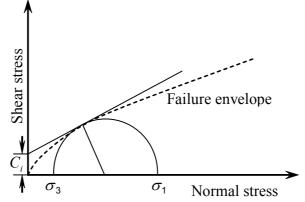
Figure 7: Schematic graph showing the definition of the instantaneous cohesion of rock joint ( $C_i$ ) in
