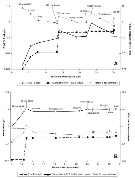
Figure 2: Total iron load and concentration profiles in the River Gaunless under low flow (Fig 2a) and high flow (Fig 2b: updated from Younger, 2000) conditions. (Note the differing horizontal axis in the two plots).
