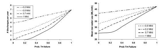
Figure 4. The effect of failure of desalination treatment on discharge (left) and mean raw water use (right) from the worked water reservoir as a function of the treatment intensity.
