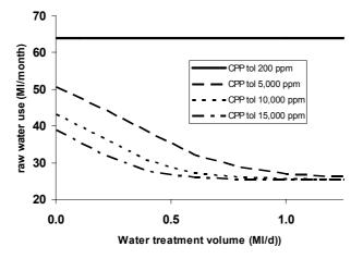
Figure 3. Raw water use with increasing water desalination volume, for a range of CPP salt tolerances. Skills
