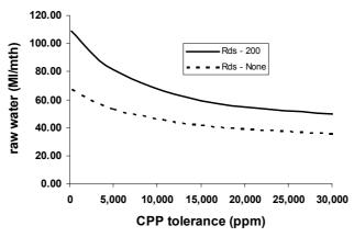
Figure 2. Raw water use with increasing salt tolerance in CPP for the case of no salt constraint for road water watering and raw water (200ppm) required for road watering.
