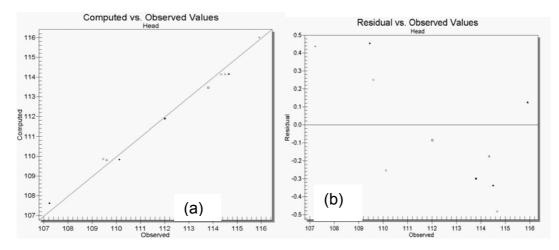
Figure 2: Steady state calibration showing (a) computed versus observed groundwater heads (mAOD) and (b) residual versus observed groundwater heads (mAOD)
