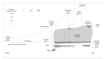
Figure 2: Conceptual cross-section of mine dewatering
