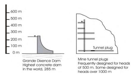
Figure 1: Comparison of Highest Dam to high Head Plugs [1]
