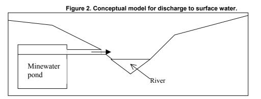
The flows calculated by GRAM for the Treeton and Silverwood ponds (Table 1) are mixed with the flow in the River Rother and River Don. PHREEQC was applied as a batch-reaction model by taking the volume of flow in a fixed time period (e.g. 1 second) and mixing the two waters together. It was assumed that the minewater and river water completely mix, and that equilibrium was instantaneous. It is recognised that both these assumptions are simplifications but are deemed appropriate for this study.
