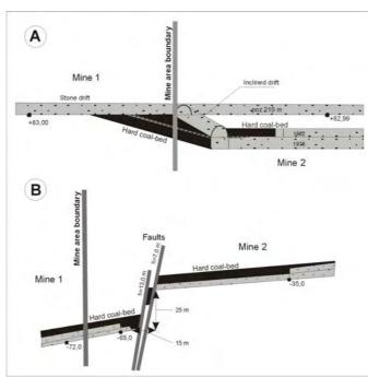
Figure 2: Exemplary of the direct (A) and indirect (B) hydraulic connections between the hard coal mines
