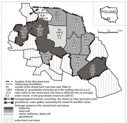
gravitationally led away to the neighboring active hard coal mine through a specially made for this purpose hydrogeological borehole, 600 mm in dimension and 129 m long to (Fig. 4).
