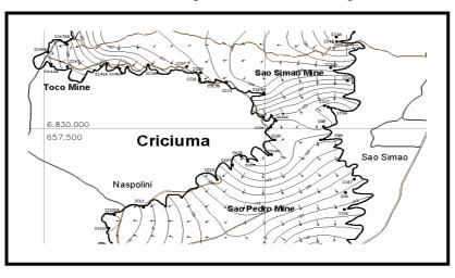
Figure 03: Map showing structural model of Barro Branco coal seam floor and flow directions inside the mines.
