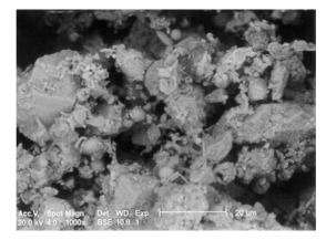
Fig 3. Electron Micrographs of Anodic slime Particles.
