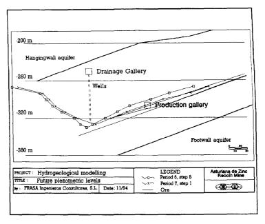
Figure 3. Mine drainage proposed at Reocín Mine, Spain (FRASA, 1994).
