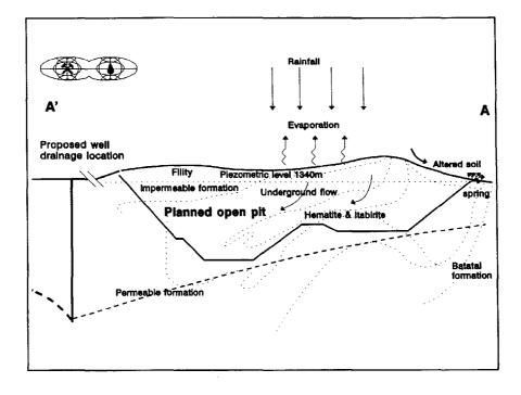
Figure 7. Schematic transversal geological cross section and proposed drainage system (FRASA, 1995).
