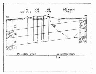
Fig.2 Schematic hydrogeological cross - section (adapted from J.Fiedler 1993).1 - crystalline bedrock; 2 - Cenomanian water-bearing system; 3 - Lower Turonian aquitard; 4 - Middle Turonian aquifer; 5 - piezometric surface of the CWBS; 6 free level of the MTA.
