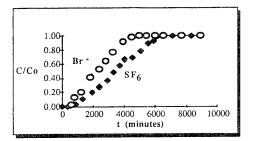
Figure 4. Break-through curves of Br<sup>-</sup> (empty polygons) and SF<sub>6</sub> (filled polygons) as observed at the pumped drain tile. Concentrations of each tracer measured (C) are relative to the steady-state concentration in the pond ( $C_0$ ). See Figure 2 for the location of the pumping well.
