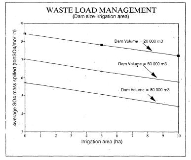
FIGURE 6.3(b) - INFLUENCE OF DIFFERENT EVAPORATION/STORAGE DAM SIZES AND IRRIGATION LAND AREAS ON THE SULPHATE LOAD DISCHARGED TO THE ENVIRONMENT
