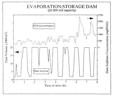
FIGURE 6.2 - WATER VOLUME AND CONCENTRATION OF A 20 000 m<sup>3</sup> EVAPORATION/STORAGE DAM OVER AN 8 YEAR MINE LIFE
