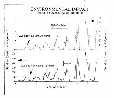
FIGURE 6.3(a) - EFFECT OF A 20 000 m<sup>3</sup> EVAPORATION/STORAGE DAM ON THE SULPHATE LOADS DISCHARGED TO THE ENVIRONMENT.
