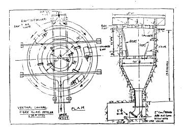
The settler is 19.8 metres deep and 12.3 metres in diametre. The capacity is approximately 1600 cubic metre and the flow rate is 48,300 cubic metres per day. The theoretical rentention time is 48 minutes.
