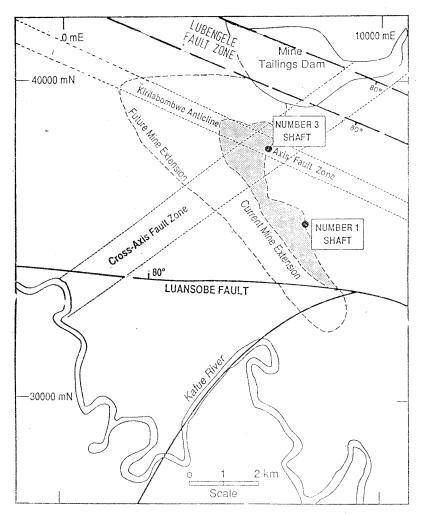
Fig. 4.1 : Map of Konkola Mine showing the faults, river, dam, and approximate limits of mining
