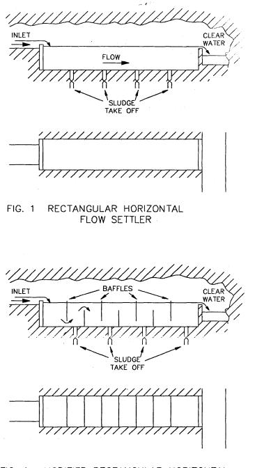
FIG. 1a MODIFIED RECTANGULAR HORIZONTAL FLOW SETTLER
