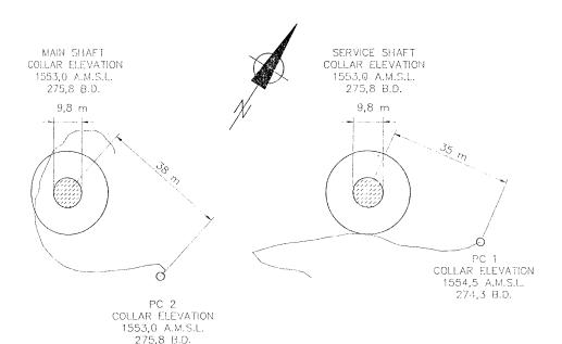
WESTERN DEEP LEVELS LIMITED ELEVATION SHOWING SHAFTS AND PC1 AND 2 BORE HOLES
