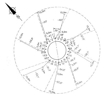
COVER HOLE DATA REQ. DIP -50° REQ. DEPTH 15,0m REQ. SPIN 35°
