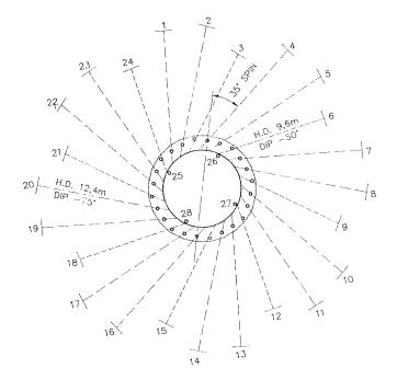
35° SPIN ON HOLES 1-24 8 HOLES 15,0m DEEP 40° OUT FROM VERTICAL 16 HOLES 48m DEEP 15° OUT FROM VERTICAL 4 VERTICAL HOLES 60,0m DEEP
