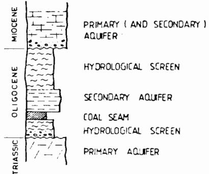
Figure 2b: Schematic geological column of the Hrastnik area.
