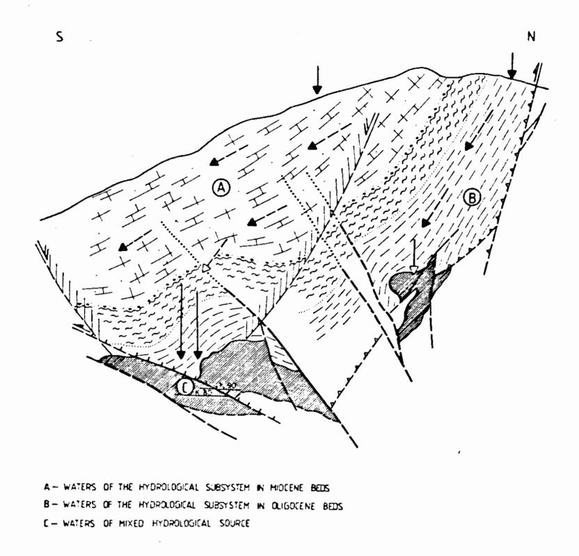
Figure 2a: Schematic geological section across the Central sector of the Hrastnik colliery.
