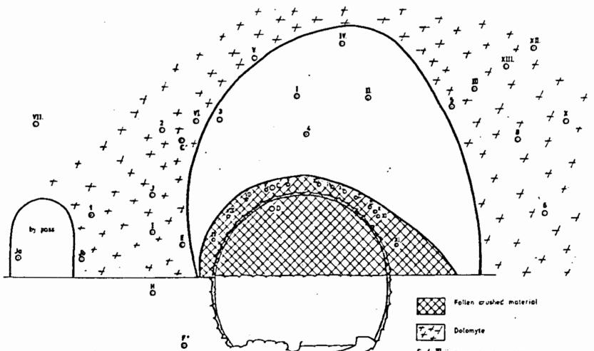
Bore holes from different phases of assanction works ŌOŌ
