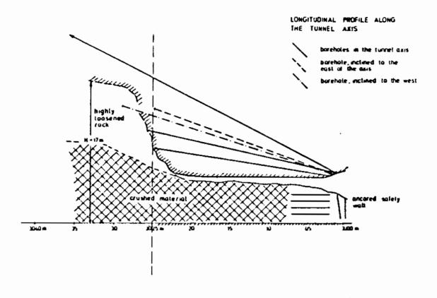
Fig.4: Longitudinal profile along the tunnel axis at the location of the second water inrush
