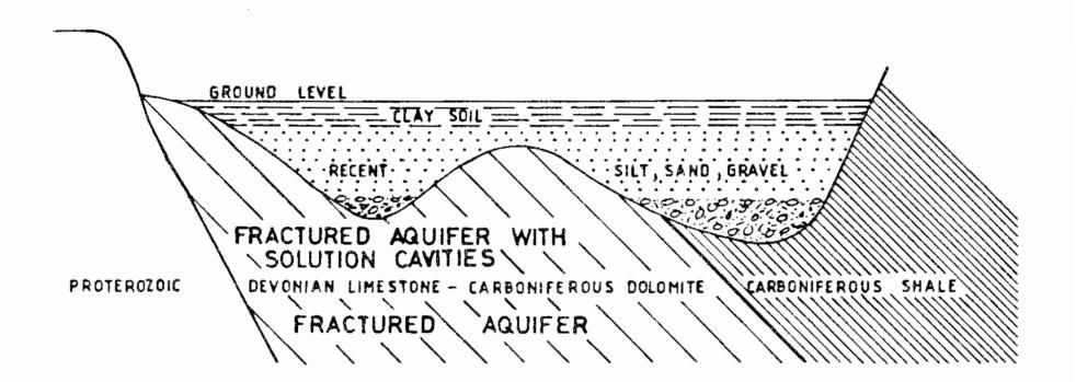
Figure 1. Diagrammatic cross-section through aquifer.
