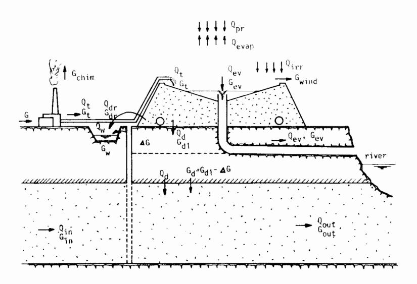
Figure 1: Transport of water and pollutant through the ash depository Transport pipes, drainage channel and the wells are actually on both sides of the depository
