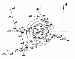
Fig. 4. Actual grout hole pattern in operation and deviation plan of central air shaft of a colliery in Shangdong
