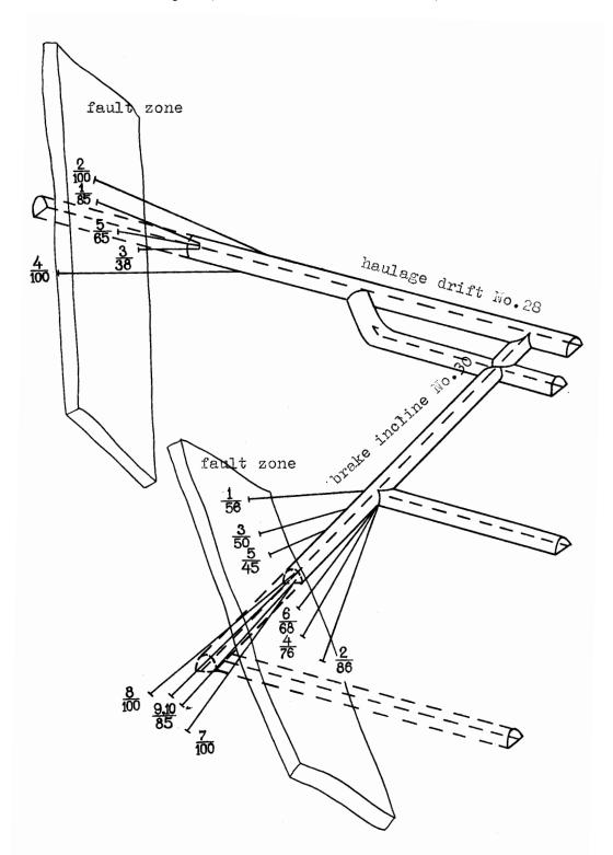
Fig. 2 Pregrouting procedure in driving deve-  ${\color{red}8}$  lopment workings
