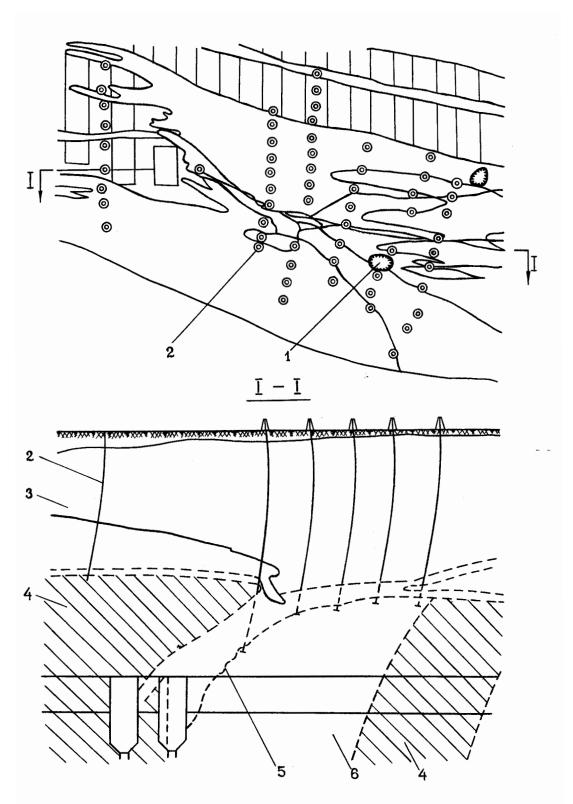
Fig. 4 Grouting scheme used during restoration of productive chambers at Stebnik Potash Plant
