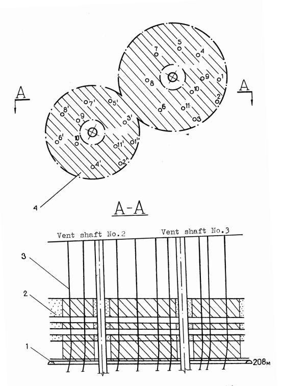
Fig. 1 Grouting procedure for abandoned workings around mine shafts of the Yuzhnaya Mine 1-water-logged abandoned workings, 2-water bearing strata, 3-grout holes, 4-grout cover
