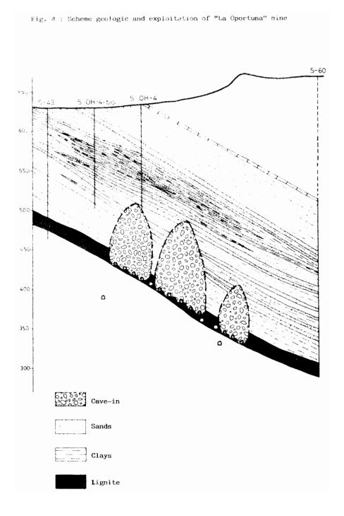
With these data a conclusion was made: the exploitation width is the parameter that controls the water floods, and when it reaches 40-50 m. the flood is produced.
