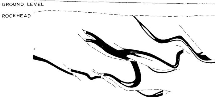
Fig.1 - Section of Big Seam through Llannon Disturbance
