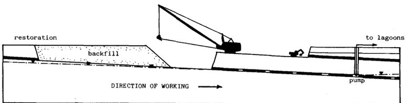
(c) SHALLOW DOWN-DIP METHOD USING LARGE DRAGLINE
