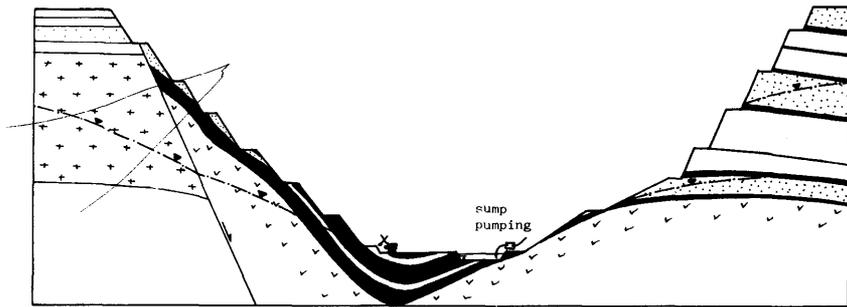
(a) DEEP OPEN PIT OPERATION USING TRUCK AND SHOVEL METHOD
