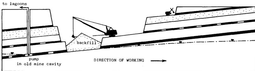
(b) BOX-CUT AND UP-DIP (RETREAT) OPERATION USING MEDIUM SIZE DRAGLINE AND TRUCK AND SHOVEL METHODS
